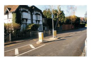
New pedestrian refuge islands will be provided, and existing refuges will be upgraded. Tactile paving will be provided where it is missing to assist pedestrians with impaired vision.
